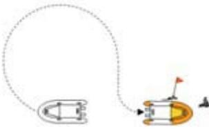
The need to keep a visual reference on the floating datum or wake means that this method needs a relatively small turning circle to be effective.
