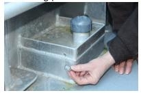
Open Fuel Tank by Removing Cap
