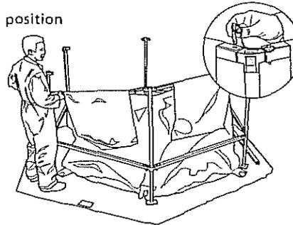
**4 .** Slide top beam under coloured fabric and connect one end to top of upright. Insert pin to lock, as in 2. Repeat to complete assembly.
