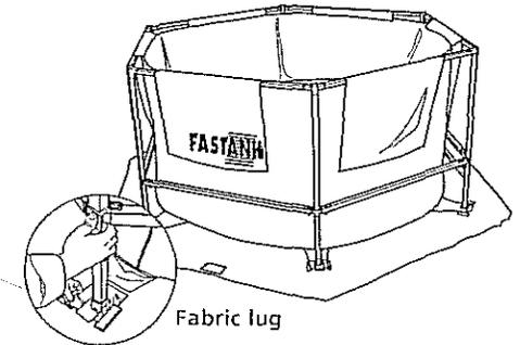
**5 .** Pull base of tank into circular shape, ensuring no wrinkles in the floor. Raise foot and loop lug strap into position as shown. Start filling tank, regularly check progress and ensure all fixings are secure.
