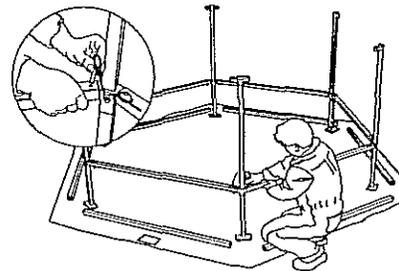
**2 .** Fix the bottom beam onto the upright and insert pin to lock. Repeat with all bottom beams
